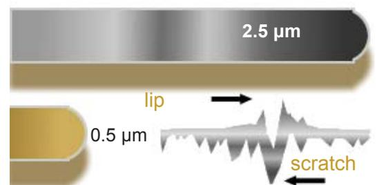
Fig. 13: Height of lip of scratches
