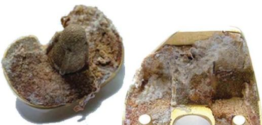
Fig. 18: Bone ingrowth in TiN coated CoCrMo knee replacement components
