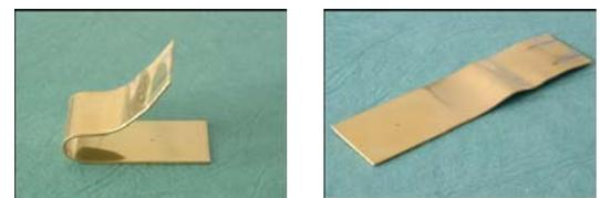
Fig. 22: Bending test to prove adhesive strengths
