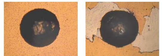
Fig. 21: Two PVD coated implants with different adhesive strengths
