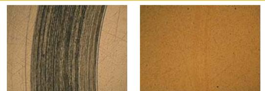
Fig. 24: Pin-on-Disk test of PMMA on TiN coated substrate.
