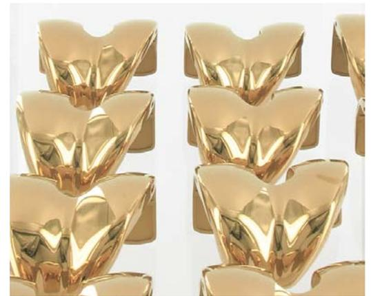
Fig. 20: TiN coated components
