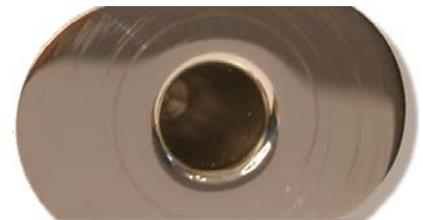
Fig. 12: Scratched non-coated CoCrMo tibial component
